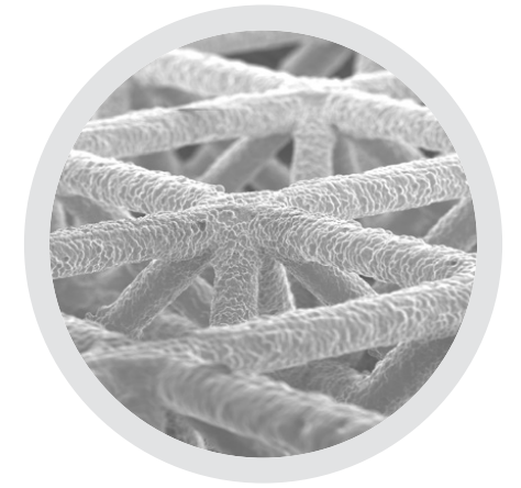
A microscopic view of a microtruss coated in a thin sleeve of nanocrystalline metal.
