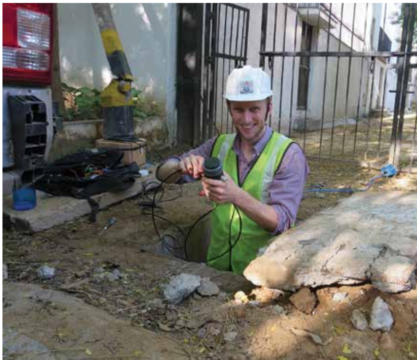
Professor David Taylor checks on his pressure, flow, and turbidity sensors in a valve chamber in Delhi, India. (Photo courtesy David Taylor)
