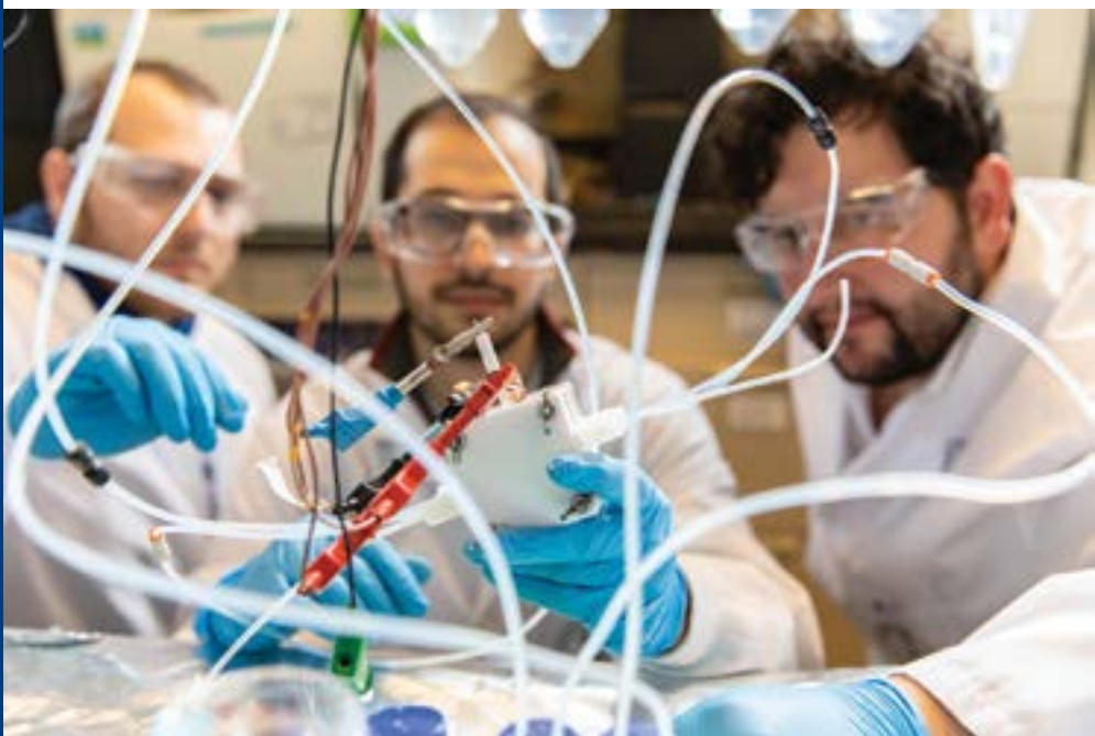
Left to right: PhD candidates Adnan Ozden, Joshua Wicks and postdoctoral fellow F. Pelayo García de Arquer operate an electrolyzer that converts CO 2 to valuable products 10 times faster than previous versions. (Photo: Daria Perevezentsev)
