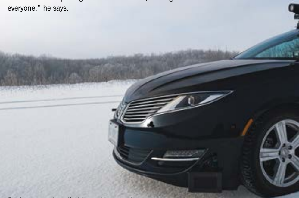
The Autonomoose is a self-driving car that was used to create the world's first dataset of driving under harsh winter conditions. (Photo courtesy University of Waterloo)
