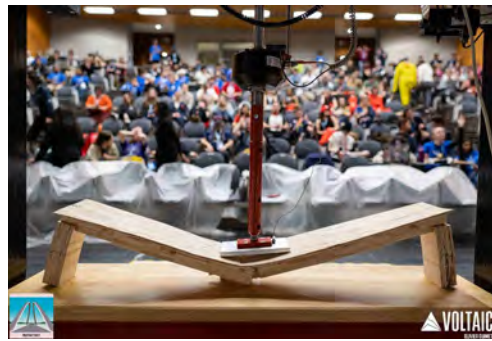
One of the UofT Bridges being tested under the hydraulic press at Concordia University
