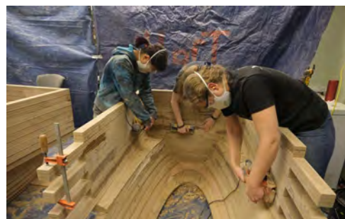
Lindsay Wells and Maggie Ye preparing the mould for the carbon fibre layup
