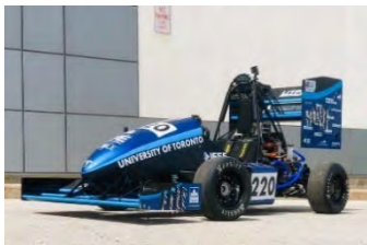
UT23, our first running electric vehicle and first driverless capable vehicle.
